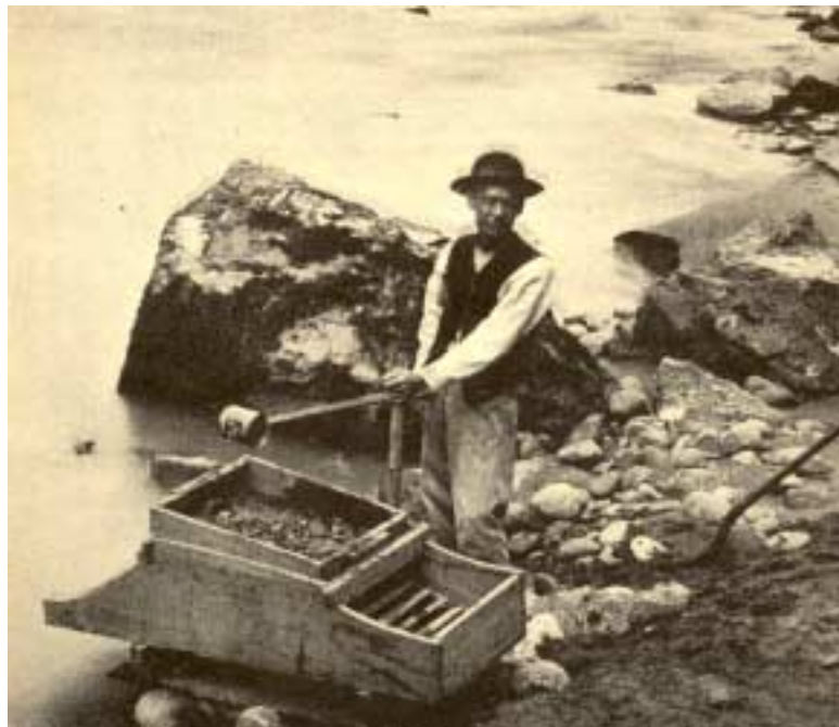
Figure 11. Chinese miner, panning for gold on the riverbed. Chinese miners invented the gold separating rocker table shown here (Taylor, 1978)
