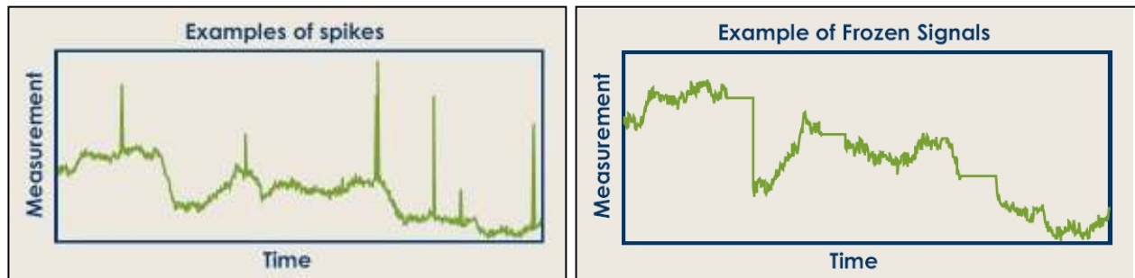
Figure 9B-9: Detection of faulty data in measurements taken within a concentrator. On the left, "spikes" can be seen in data that are artifacts or sensor failures. On the right, the output shows signs of "frozen" signals in which an output remains unchanged over a period of time indicative of a sensor or sampling failure.
