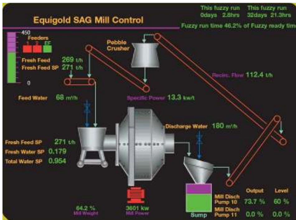
Figure 9B-2a. Grinding circuit showing control systems in use with a SAG mill circuit and a downstream second stage ball-milling.
